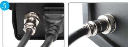
Plug one end of the circular 5-pin power connector into the Skylux ballast and rotate the silver ring clockwise on the cord connector to secure the cord to the metal ballast. Plug the opposite end of the cord into the rear connection point on the Skylux and rotate the silver ring clockwise to secure the cord to the back of the unit.
